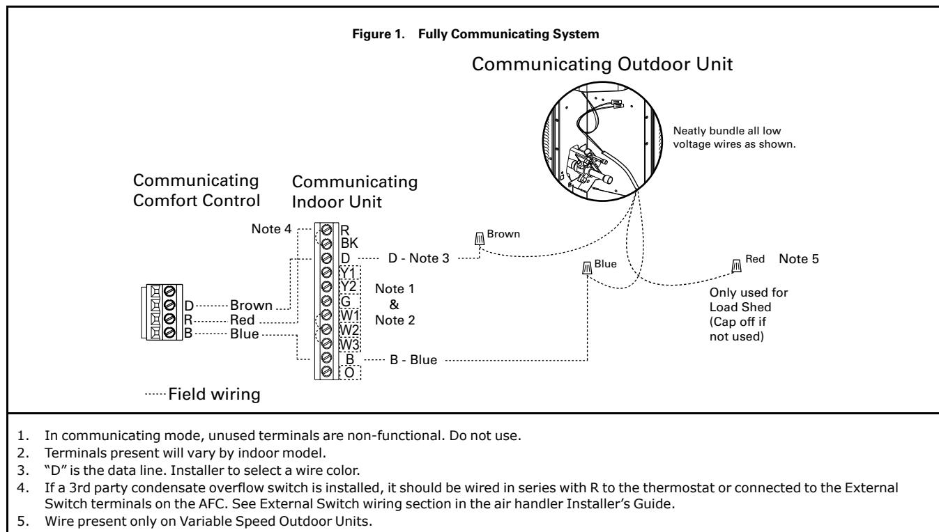
**Note:** Anti-oxidizing grease is supplied in the documentation package for use when making low voltage field wiring connections at the outdoor unit. Apply grease to field wiring before installing wire caps to protect these connections from corrosion.
