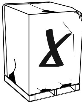
2. To remove the unit from the pallet, remove tabs by cutting with a sharp tool.
