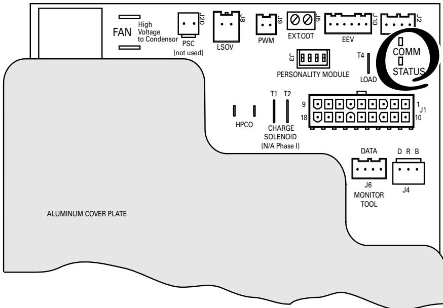
The Status (Green) and COMM (Amber) LEDs are located in the upper right region of the Control Board.
